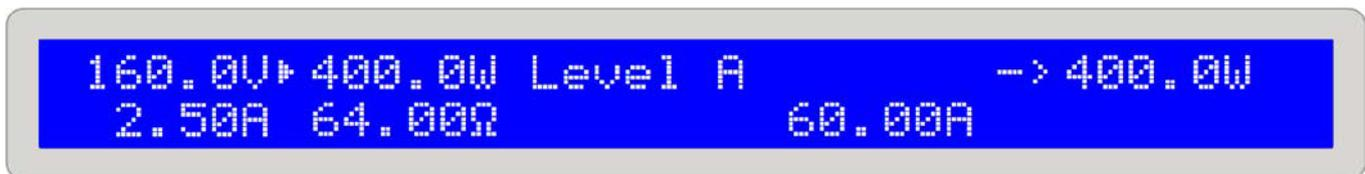
Figure 9. Normal load operation in CP regulation mode
