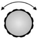
This rotary knob has no end stop. With every position **Setting (6)** changes the set value resp. the parameter (in the setup menu) which was chosen before by **Selection (5)**.
